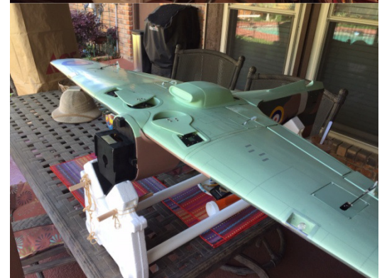
Above photos show gear and flap installation before/after attaching outboard wing panels
